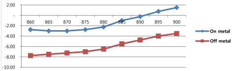
•Fastener reads longer by 23% off metal (or on non metal surface). It can be applied for BOTH metal and off metal application.
