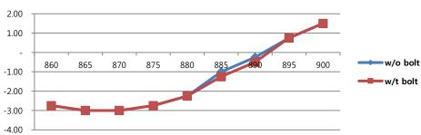
•Fastener reads same, regardless of whether it is fastened with metal bolt in two holes (located on center of both ends) or not. Stainless steel M4 bolt with round head is best fit for Fastener.
